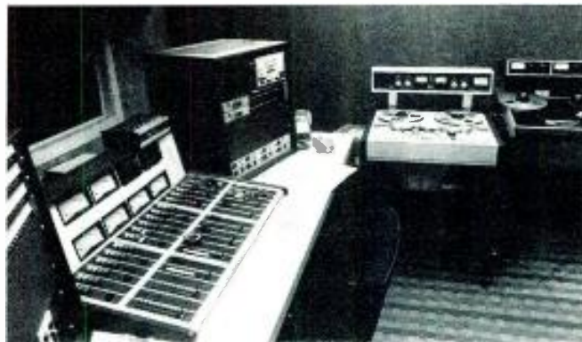
Studio control room B. The stereo phase meter (center) helps the operator keep phasing within one degree
