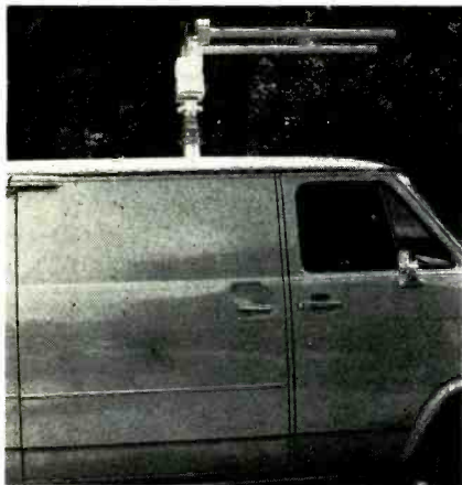
Fig. 1. The Golden Rod™ from Nurad and (Fig. 2, right) the Disc Rod™ from MAC were designed to provide high gain and low wind loading
