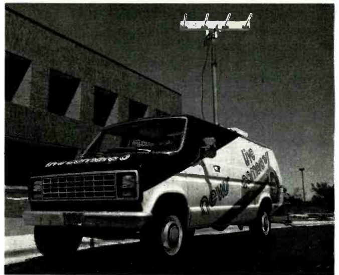
Fig. 1. The Golden Rod™ from Nurad and (Fig. 2, right) the Disc Rod™ from MAC were designed to provide high gain and low wind loading
