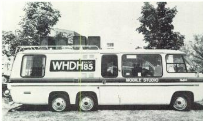
The core of an ENG operation is a vehicle, like this one at WHDH, Boston, that has a radio link to the studios. The radio link should produce signals of broadcast quality, so they can be aired as received or recorded for later broadcast
