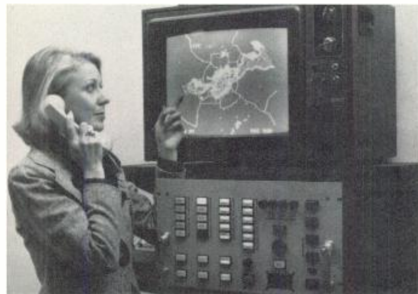
In the above photograph, the operator is seen dialing up a radar weather display on Weatheration's computer graphics system. A custom map is seen superimposed over the radar display
