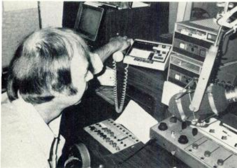
In KLAQ/KPPL newsroom, receiver for 450 MHz two way radio is on shelf, within easy reach of operator. He can put an incoming report on the air or record it on the cart machine, next to the receiver on the shelf
