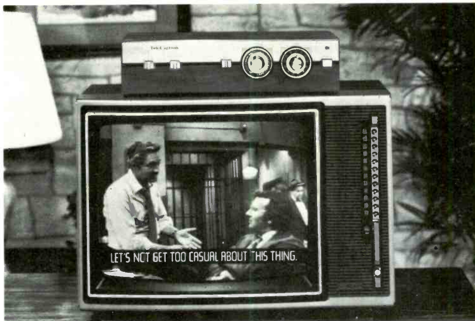
Typical television scene with closed caption across foot of screen, produced by decoder on top of television receiver
