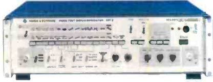
Video test signal generator SPF 2, with test line insertion
