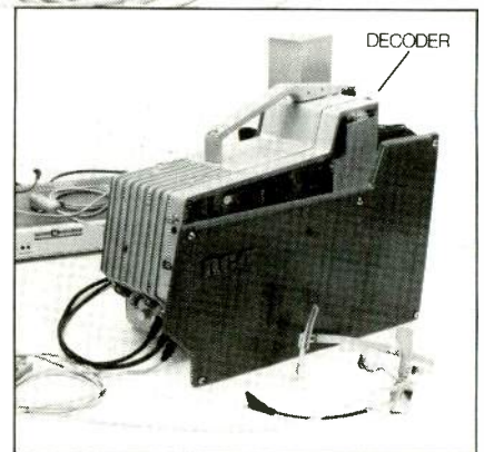
RCA TK-76B shown with decoder neatly "sandwiched" between camera body and door.
