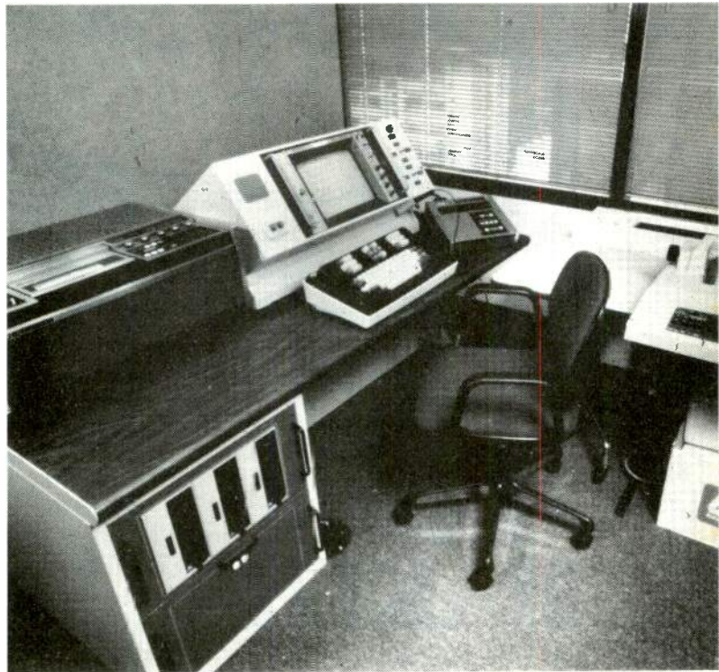
Editing system developed for putting closed captions onto television programs includes an editing console with CRT readout, electronics system converting captions into digital form, and floppy disc to hold captions and SMPTE code, for application to program
