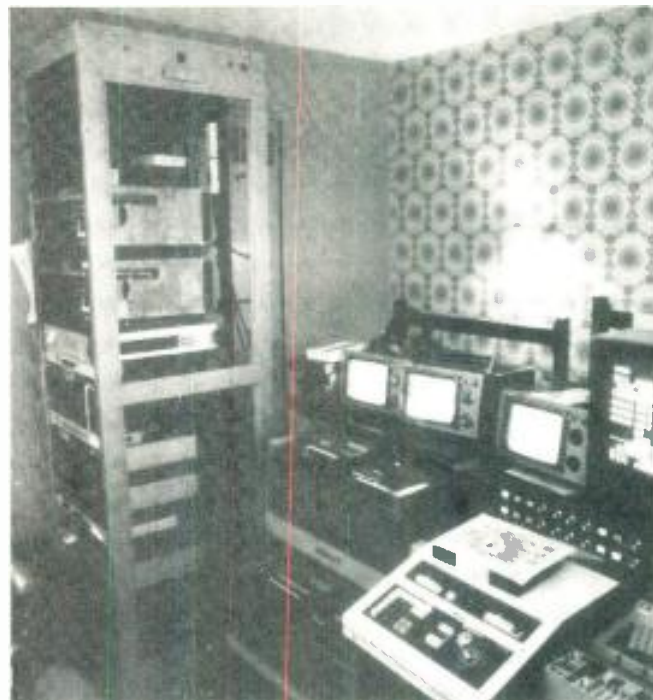
ABC's London operation was based almost exclusively around 3/4-inch equipment, including Sony BVU-200 decks. A single-channel Quantel DPE-5000 (to right of Convergence ECS-103 editor) was used for special effects.
