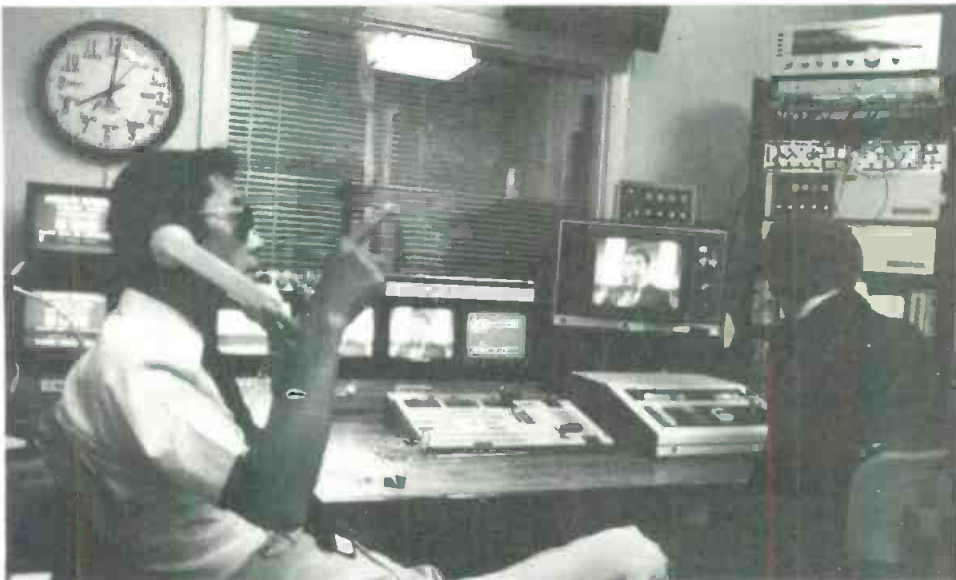
Pyramid's production/edit room at the National Press Building. A Convergence A/B roll editor is used in conjunction with ADDA VW-1 frame synchronizers.
