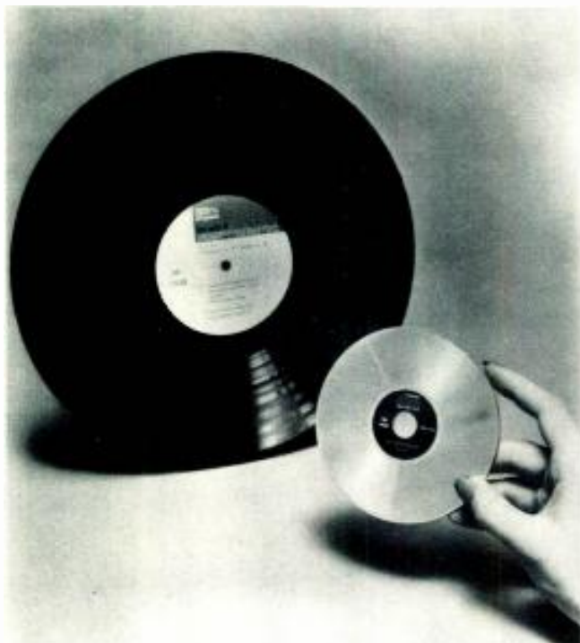
One side of the digital audio disc holds as much music as both sides of an ordinary LP, shown in background.
