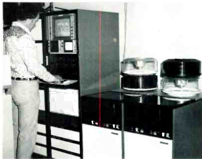
The Ampex ESS-2 relies on 200 Mbyte disk packs each of which can hold some 8000 stills. KDFW, Dallas, pictured here, has a two-disk drive system.
