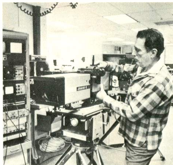
Cameraman at ABC Engineering Lab attaches a Canon J20x8.5BIE lens to camera for EFP use to undergo lens tests.
