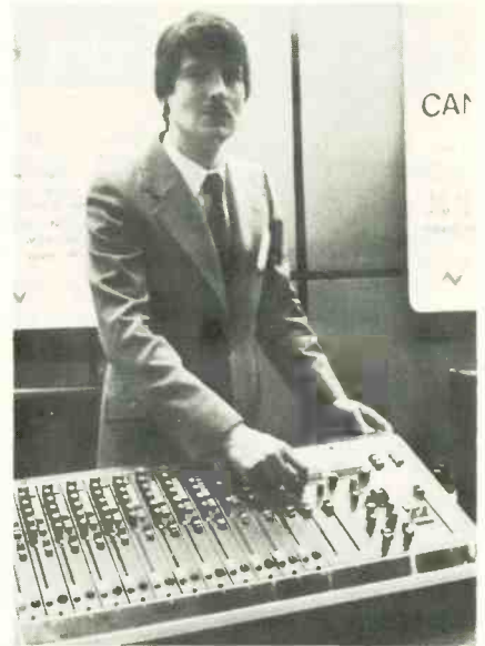
Rupert Neve's digital console is the first to use all-digital control and digital audio processing.
