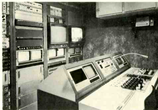
Video control room of TAV's 740 truck contains computer controls for the unit's six triax color cameras and a full complement of video monitors.
