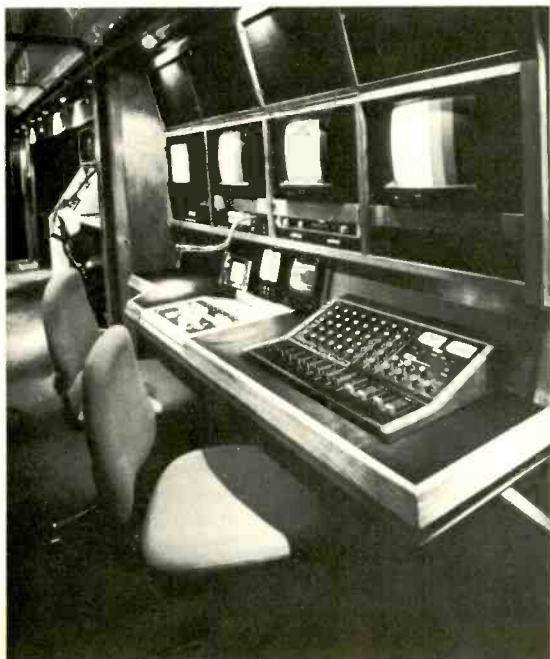
Centro's award-winning videotape truck, delivered last year to ABC Hollywood. View shows the preliminary editing/machine control area, looking aft into the tape area with its five VPR-2s.
