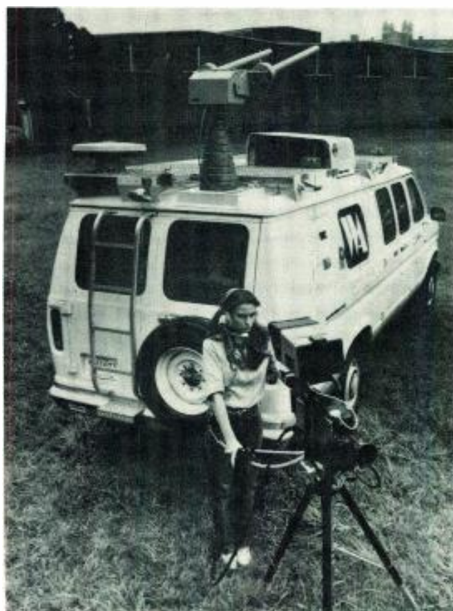
This is cable TV? Yes, it's part of the growing effort by operators to promote localism. Above is a Peirce-Phelps equipped van for Warner Amex of Mesquite, TX, shown here with Dualrod antenna by Nurad.
