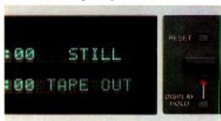
Display board for self-diagnostics and other data-processing functions.
