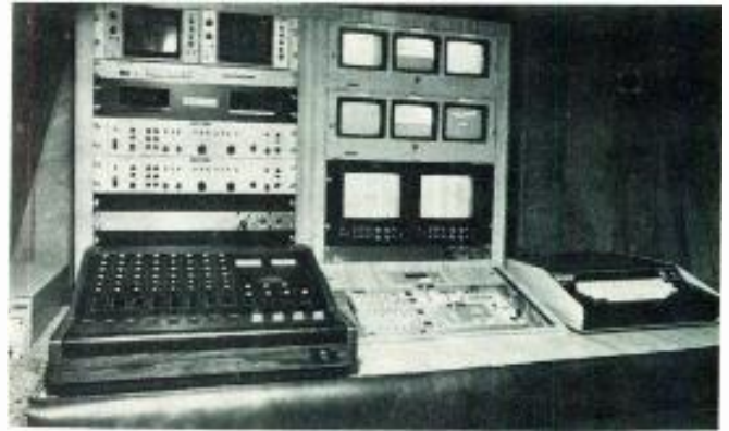
Interior of the Midwest M-20 van built for Storer Cable TV shows the broadcast quality audio and video equipment now going into local origination vans.
