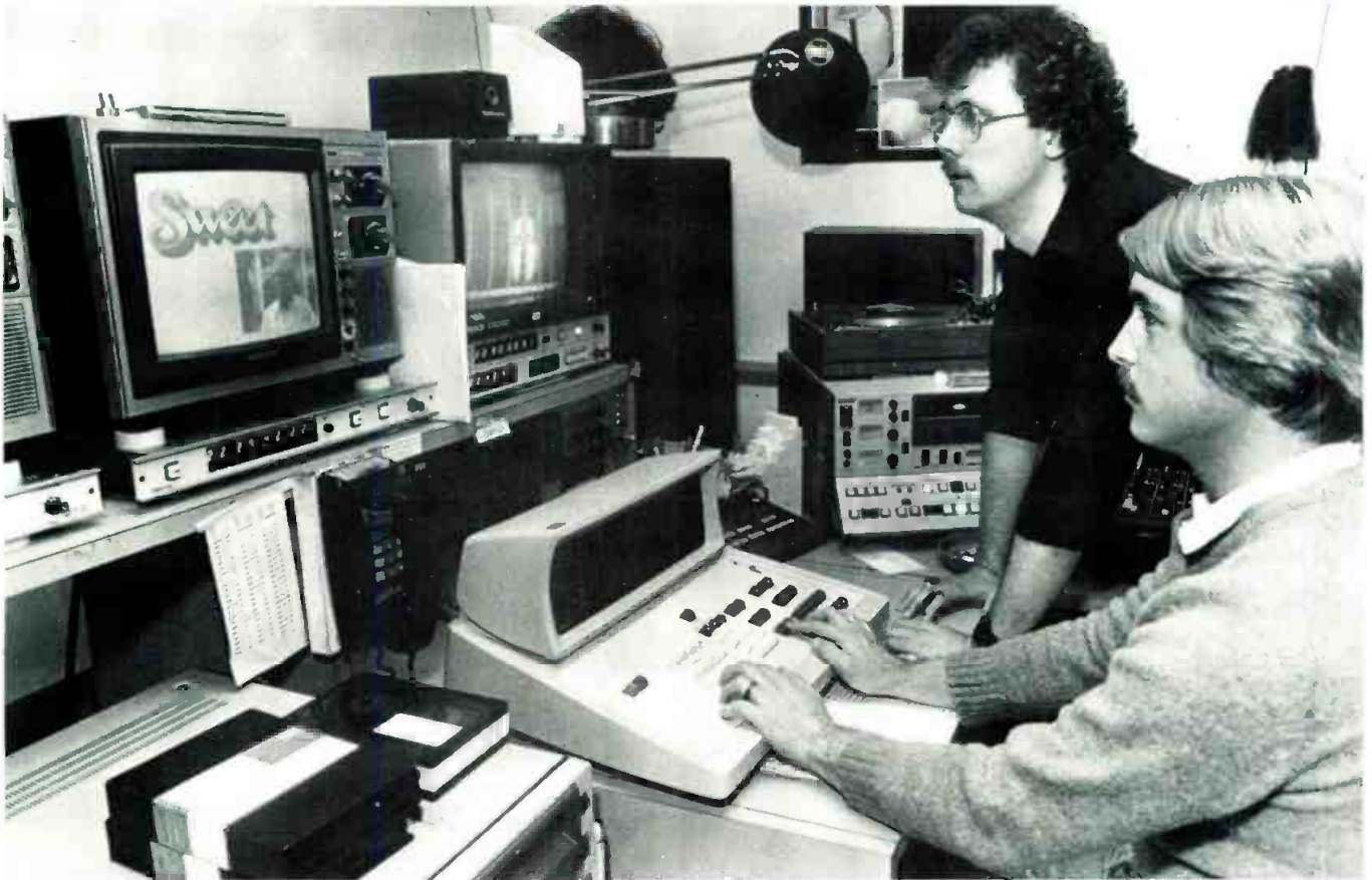
KYW producer Jim Anderson watches as Craig Ruxton operates the station's Datatron Tempo 76 editor. With the Sony BVU-800 decks, the system gives frame-accurate editing.
