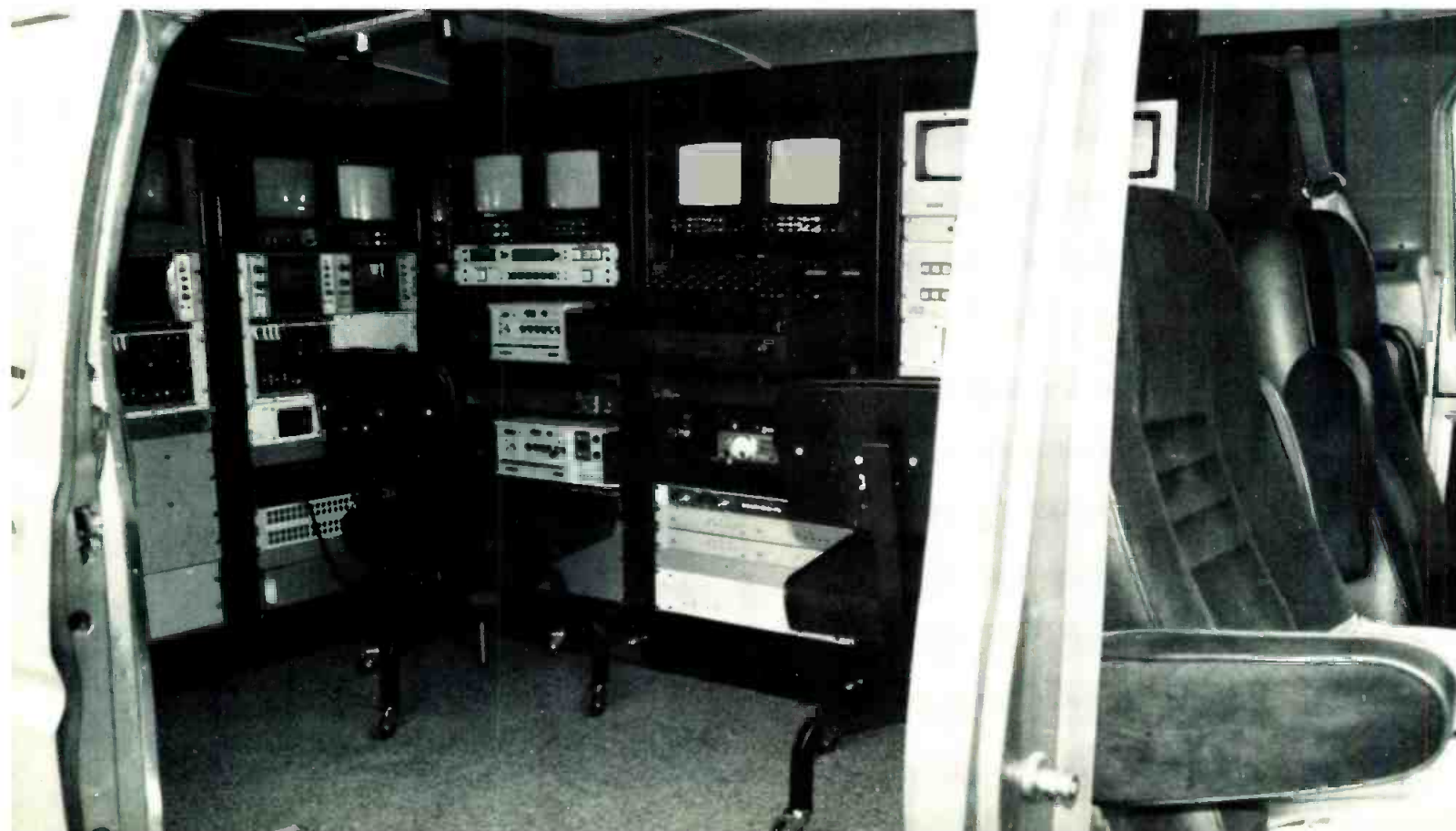
Shook's modification of the Econoline ENG van shows how two-person crew can operate console and video equipment.
