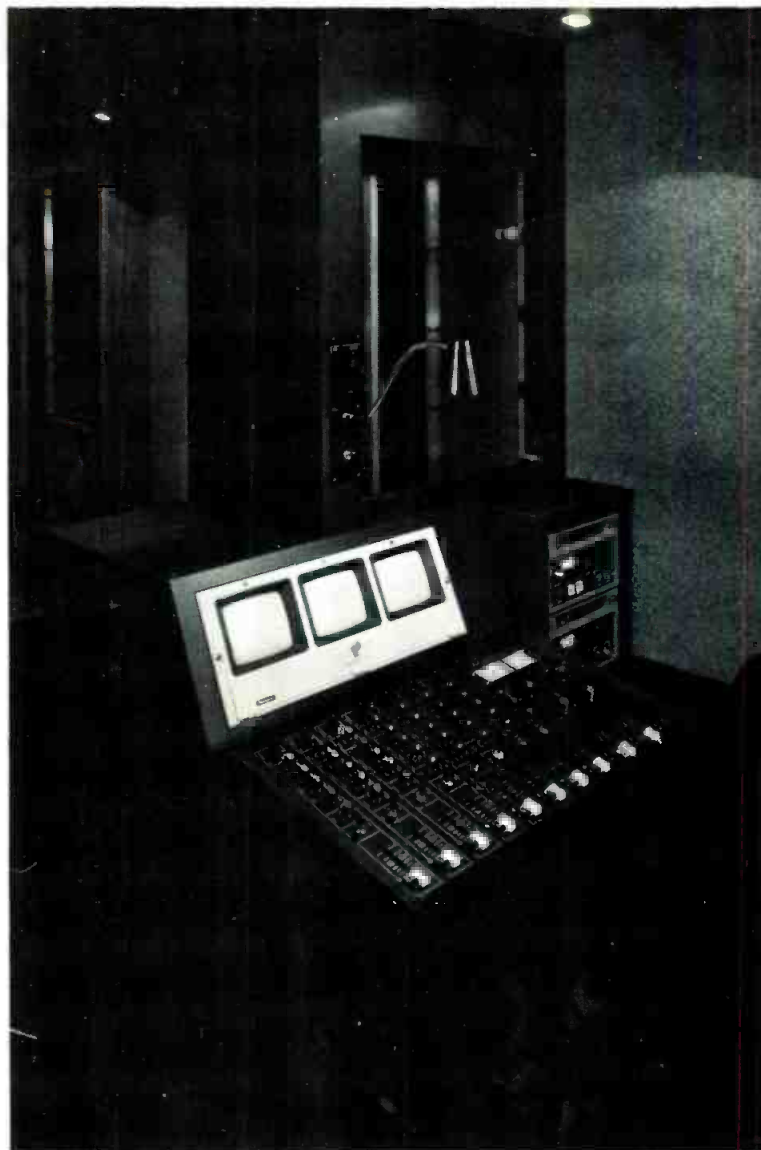
In a Wolf Coach truck, a Richmond Sound console fits next to BE carts and Panasonic video monitors.
