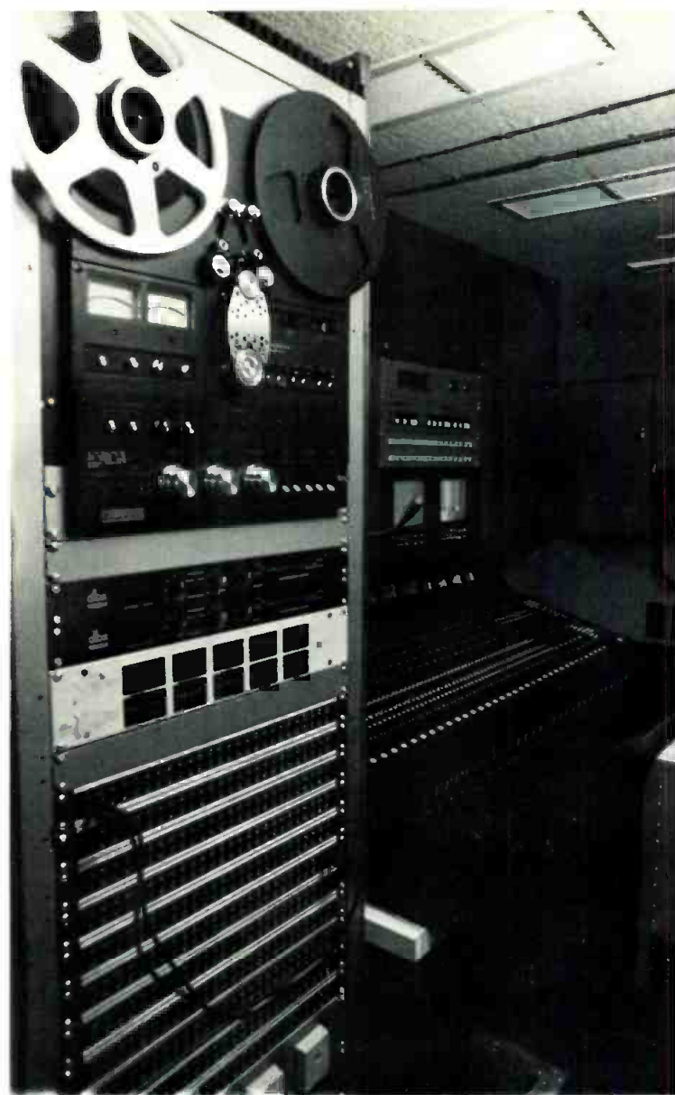
Quality Video's van by RCA shows a 32-in Yamaha console, Technics deck, and dbx processing.
