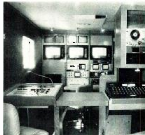
Edit bay at WJXT-TV, showing Grass Valley 1600 production switcher and Yamaha audio board.
