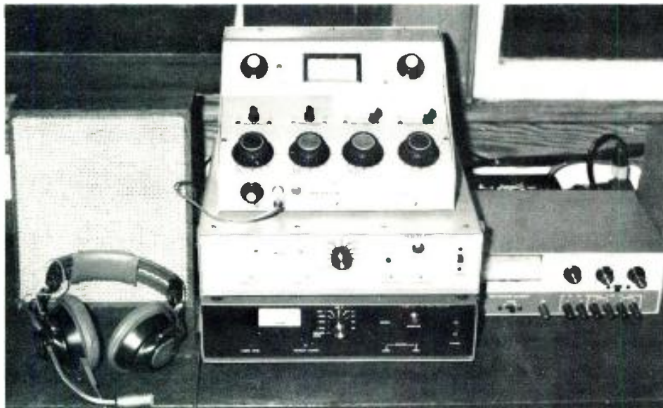
Marti receivers for 450 MHz (top) and 160 MHz (bottom) in use at KRED/KPDQ.
