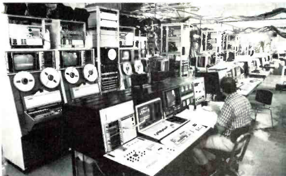
ISC editors and Ampex VPR-3s set up for "war games" trial run. Edit bays also contain Grass Valley switchers and Graham-Patten audio faders.
