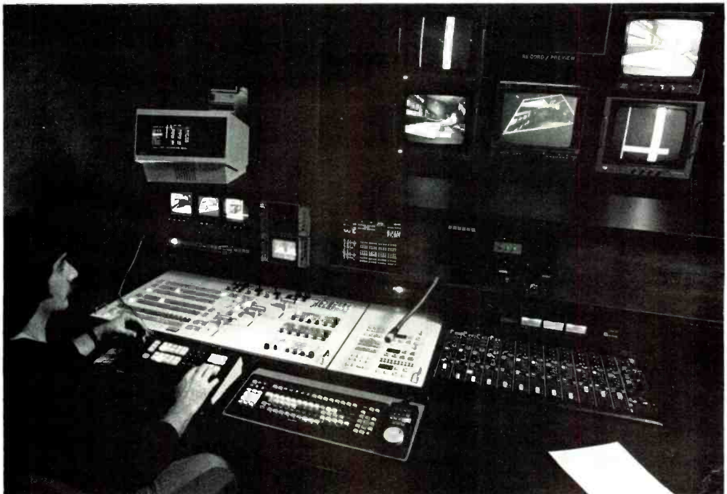
The Post Group chief engineer Rich Thorne creates effect on Ampex ADO interfaced with CMX 340X editor and Grass Valley switcher.
