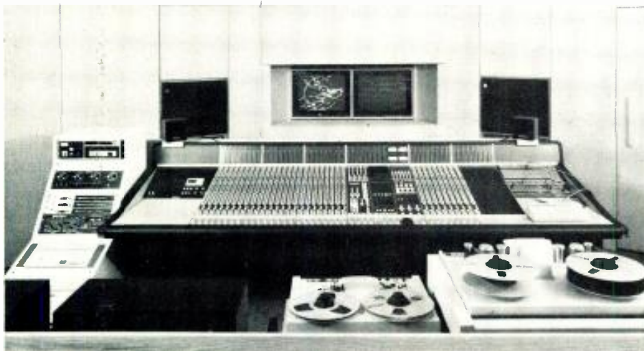
The SL6000E console from Solid State Logic with 40 inputs is the center of the CFTO-TV audio post-production room in Toronto. Otari and Ampex ATRs fill out the complement of equipment. The room is based on the live end/dead end theory and is totally symmetrical.
