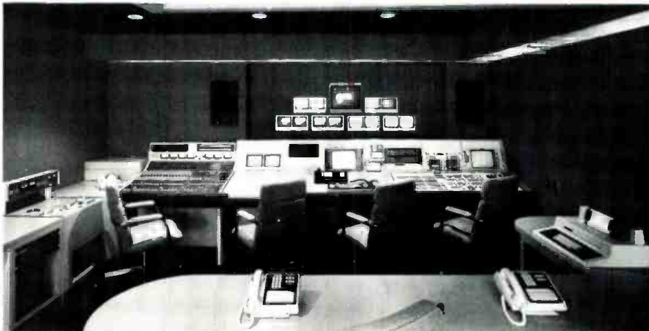
Empire's new one-inch editing suite was designed and built by AF Associates. The facility includes a CDL 1080 switcher, an Ampex ADO, Dubner CBG-1, an ADM 1600 console, and Studer A-80 tape deck.
