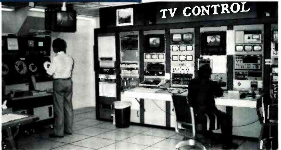
KUMV-TV control room includes Ampex VPR-2B VTRs, an American Data routing switcher, and a Grass Valley production switcher.
