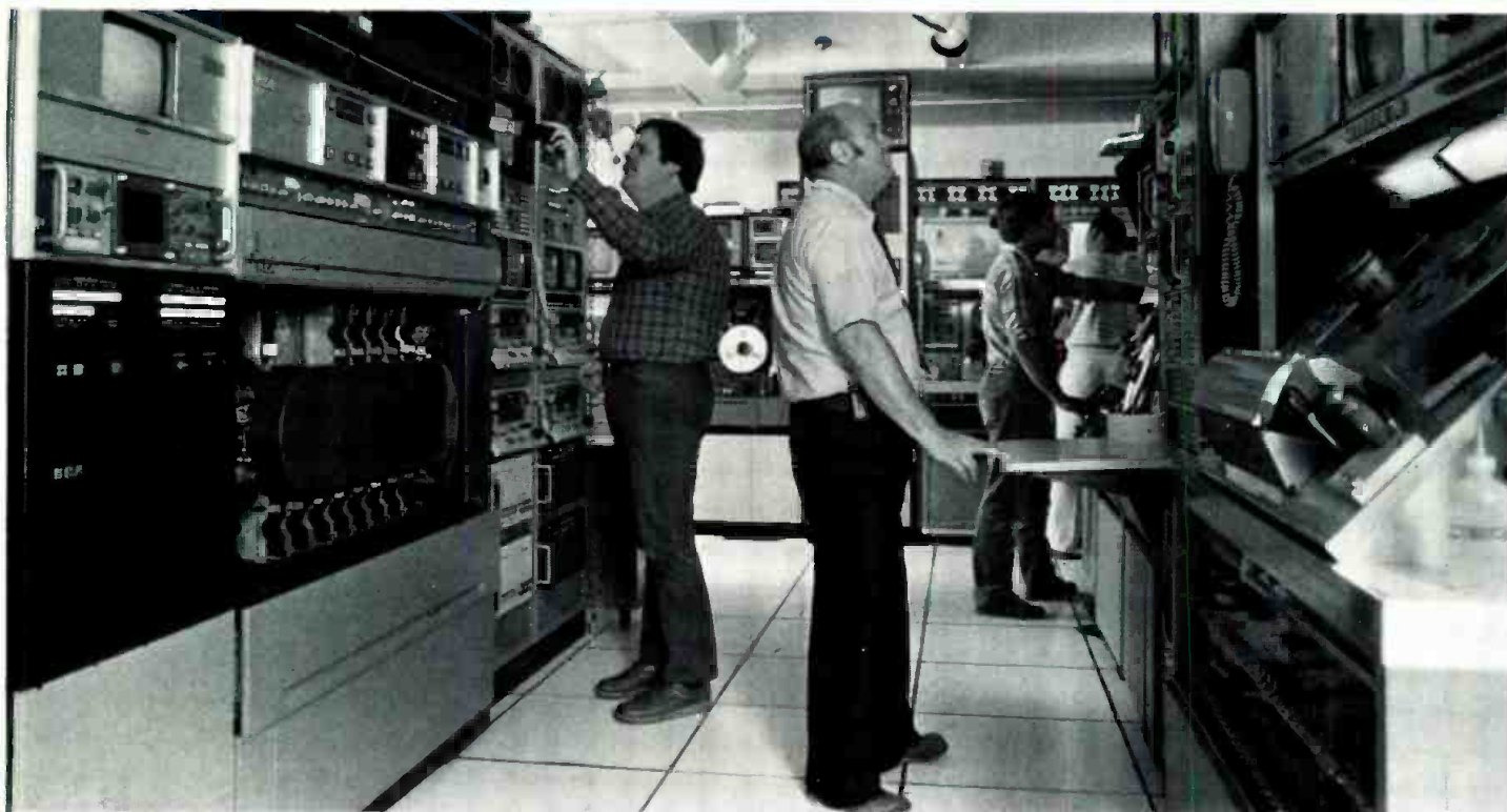
Typically busy WTVN telecine area has six Hitachi HR VTRs and RCA cart and quad decks.
