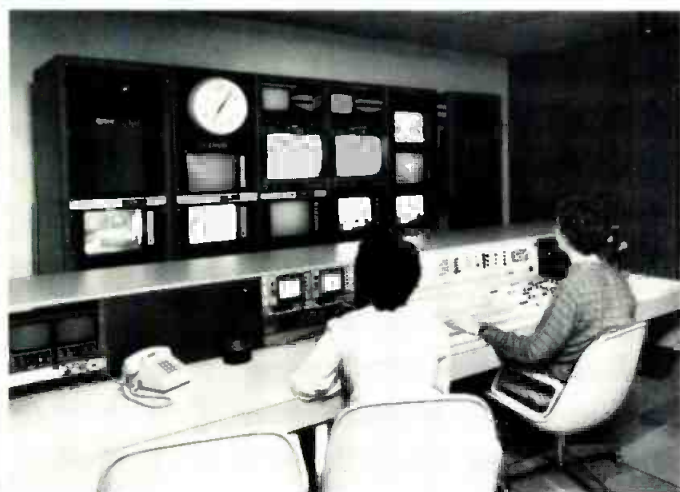
View of TV 1's Grass Valley 300-3 switcher. This large studio has 24-track audio capability, with an MCI JH-500 recorder and MCI and Ampex ATRs.
