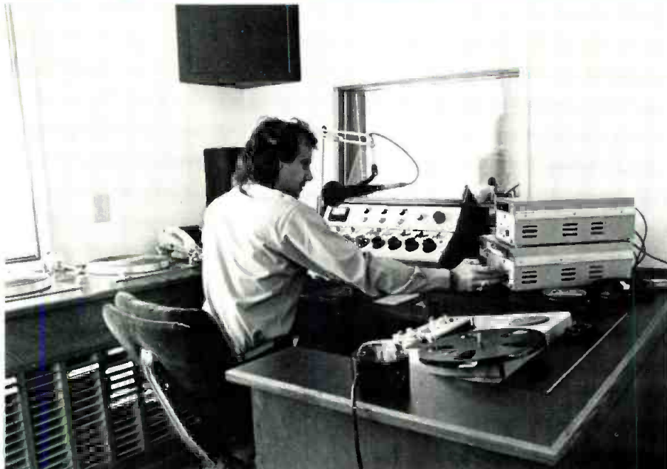
Custom-built console and Audicord cart machines are center of bright production room with turntables and cart racks to the left.
