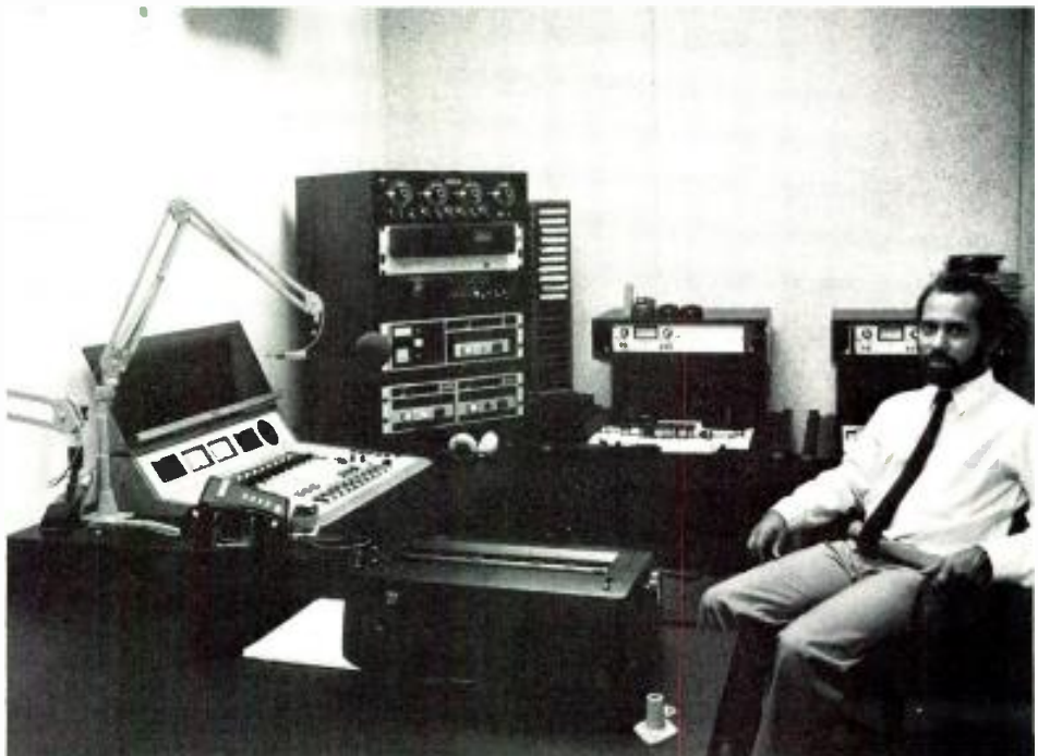
News producer Ron Bradford in Studio 1 with Pacific Recorders console, ITC carts, and MCI tape machines.
