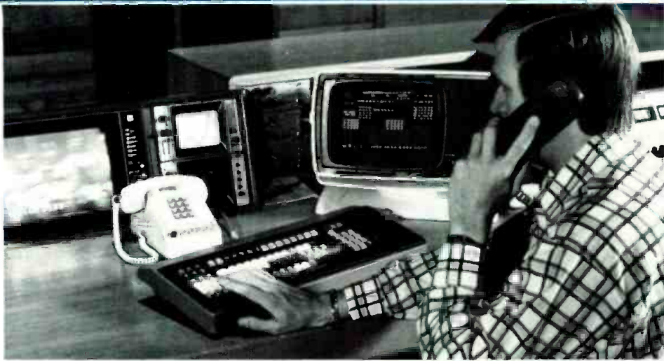
The CMX 340X keyboard and terminal shown here have corresponding CMX-1 2 intelligent interfaces located in the master control operator stations. To the right of the CMX terminal is the audio console and Grass Valley switcher.
