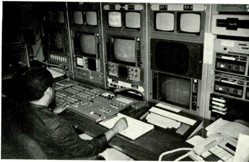
In WPIX-TV's master control room floppy disks from the traffic department are plugged directly into the station automation system at right.
