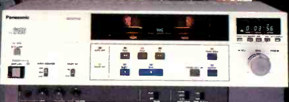
AG-6100 VHS playback deck. 14-step dial search. Frame advance, auto-repeat.
