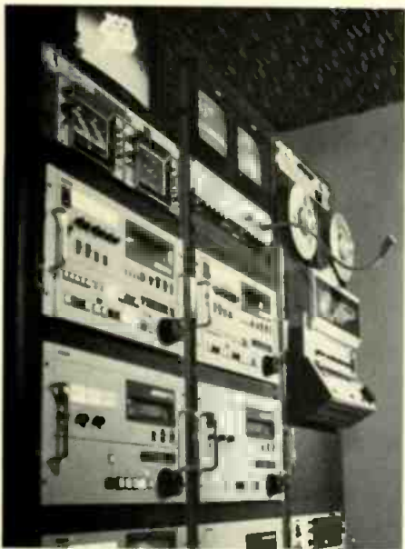
A full-service component Betacam facility, Rock Solid features a machine room with Sony BVH-2000, VCRs, and all routing and electronic equipment.
