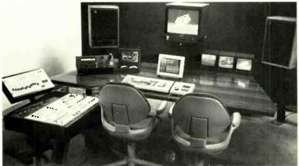
Rock Solid's Edit A contains Grass Valley component video switcher, Dubner character generator, Tannoy audio monitors, and Sony BVM-5000.
