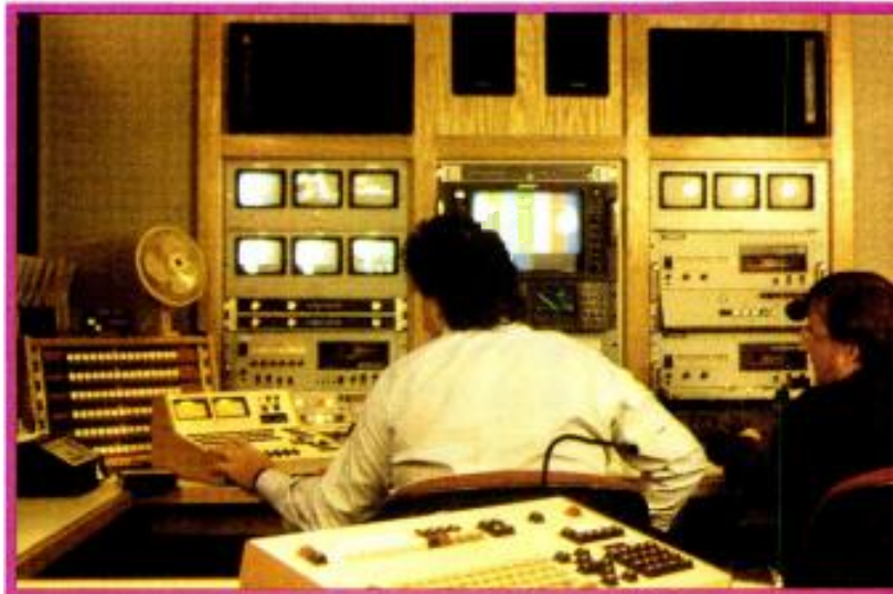
The Betacam edit suite at KIRO-TV's Third Avenue Productions, in Seattle, processes all signals in composite form for reasons of economy.
