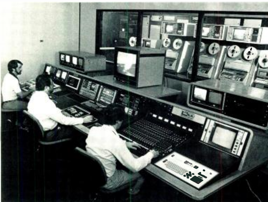
The Ampex Creative Command Center is a full-fledged studio-based linear editing system.
