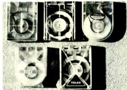
Figure 4: A collection of carts. The endless loop cartridge as it appeared over the years.
