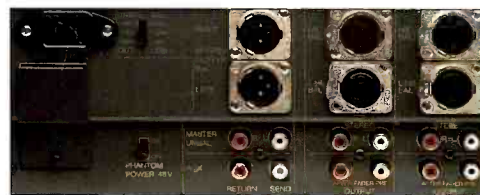
Detail of connection panel at rear of console equipped with XLR and RCA connectors
