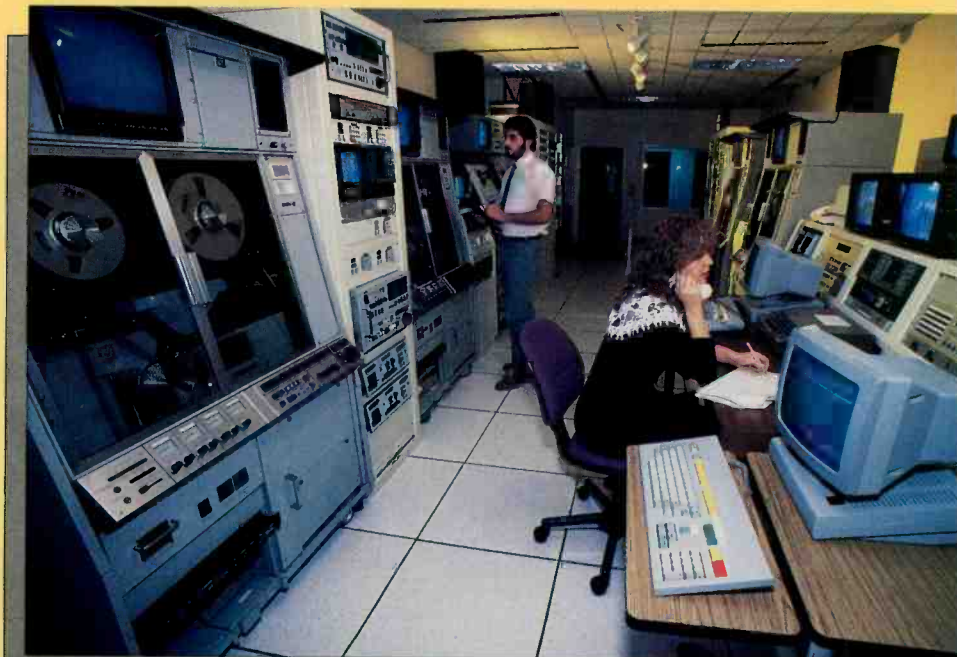
All programming and commercials air from WSYT's Lakart II automation system, which controls a mix of VTRs and ties in directly to the Columbine traffic computer.
