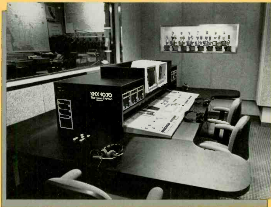
The new on-air console at KNX-AM brings everything—including the automated news system—within arms reach for combo operation.
