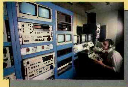
A Bosch/BTS TVS/TAS 2000 routing system interconnects master control (shown) with production control.
