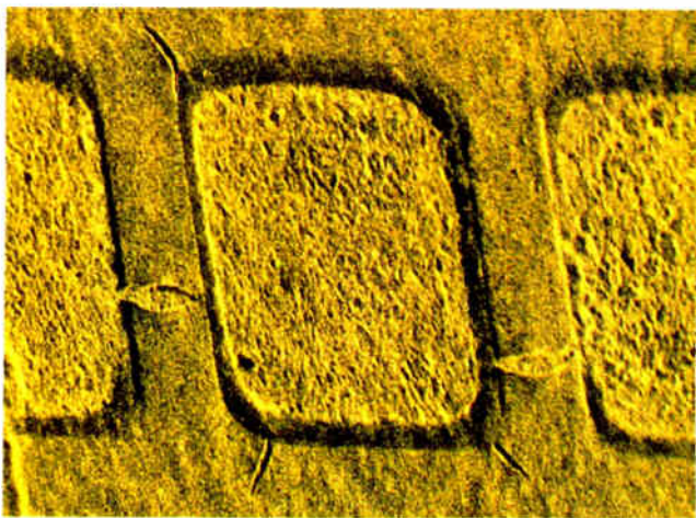
Magnified more than 500 times, the first thin-film, high-temperature superconducting quantum interference device—or SQUID—is shown here.
