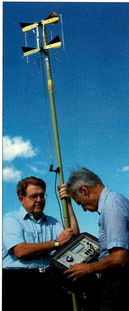
Performing line-of-sight visual-to-aural carrier ratio measurements using a directive receiving antenna and a field strength meter.
