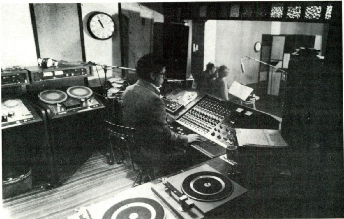
The stereo production control room is equipped with ITC 850 machines on the left and a Rupert Neve BCM10/2 mixer in center.
