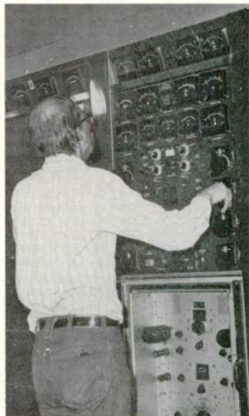
An HCJB engineer adjusts the RCA BHF-100 100 kW shortwave transmitter.
