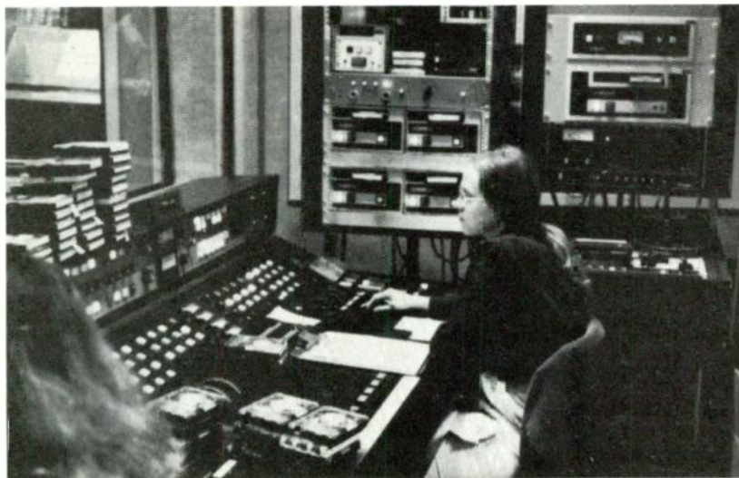
Engineering side of control room used for election-night programming. Engineer Maureen Shaughnessy at console mixes all program elements into the final air product.
