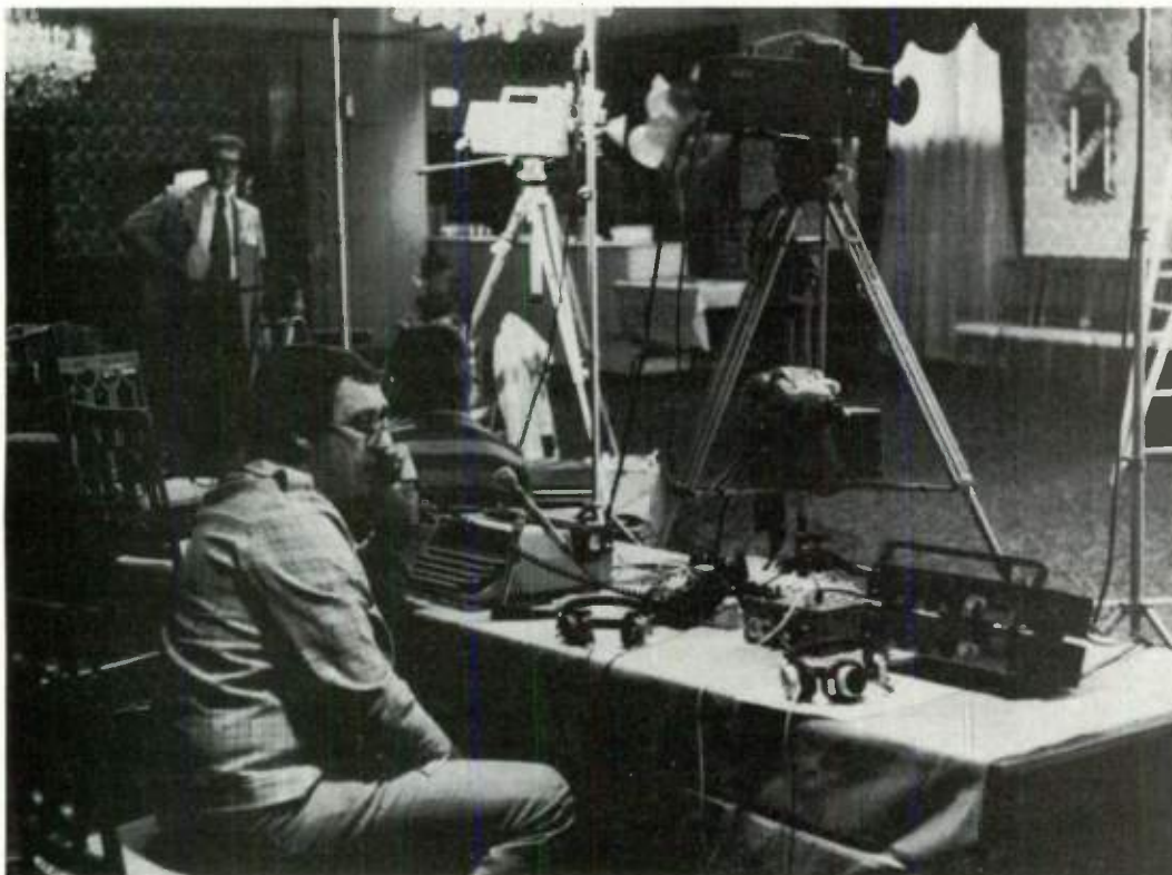
Scranton, Pa., wire remote setup with reporter Ed Kasuba. Equipment includes two "piggy-back" Shure mixers and KYW-built microphone mult box.
