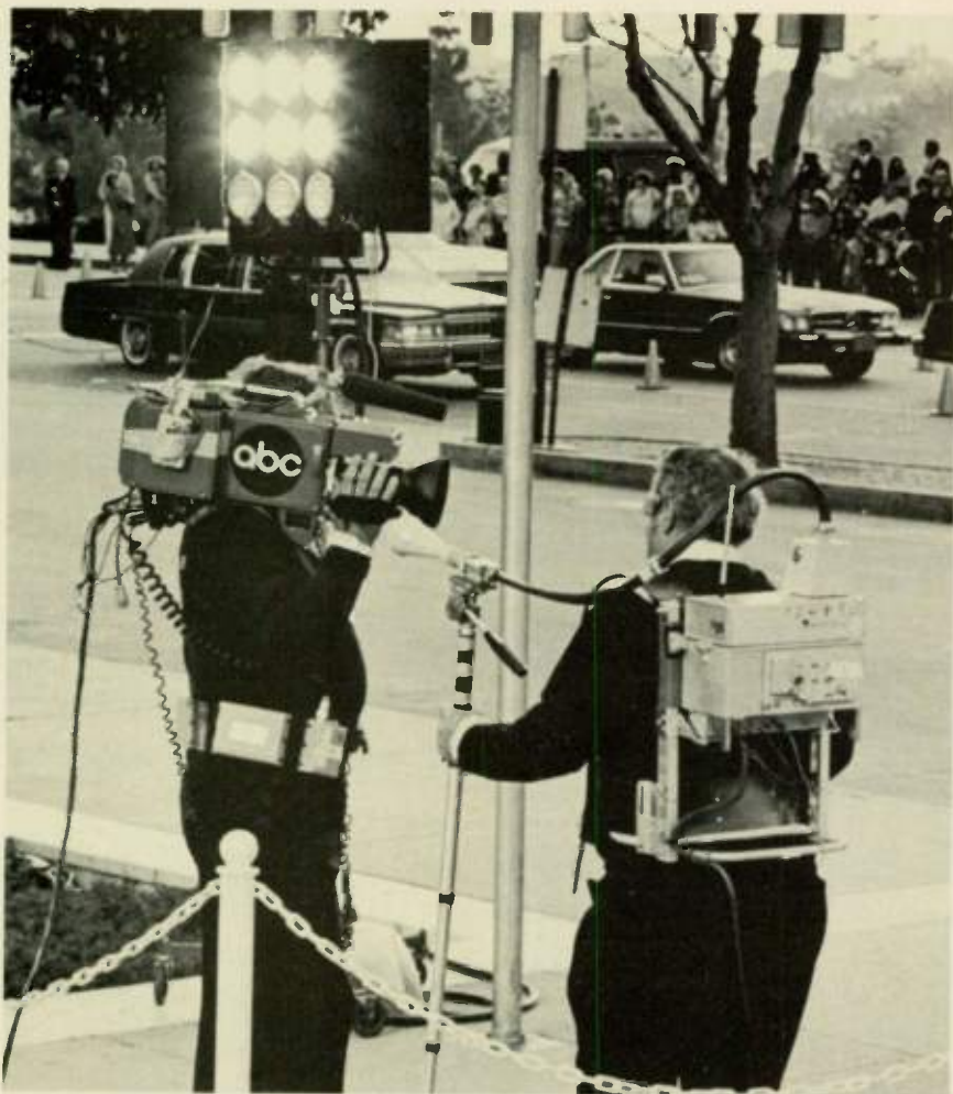
An ABC camera crew uses a special Ikegami/ABC RF camera link to get shots of arriving celebrities. These sequences were recorded and "hot edited" together immediately before the show for the opening montage.
