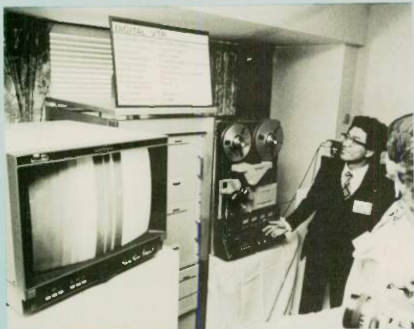
Takeo Eguchi, Sony's digital video expert, is shown demonstrating the digital VTR which his company developed using the BVH 1000 type C transport. Back to the left of the VTR contains the digital processing circuitry. Conrac's professional colour monitor with a precision comb filter displays a near-perfect test signal playback. (Photo by Donna Foster-Roizen)
