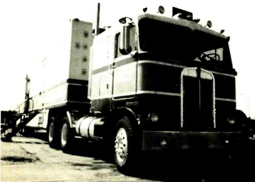
**This 18 wheeler is the Columbia's mobile maintenance facility. It includes a machine shop, night sign equipment, portable mooring mast, and spare parts supply. (Photo by Glen Pensinger)**
