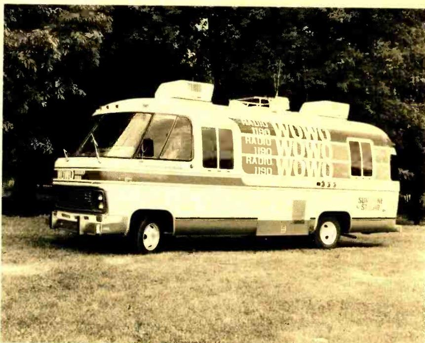
The Sunshine Studio is a customized Angosy Airstream Motor Home fully equipped with audio control and transmitting equipment. (Photo by Dennis Stierer)
