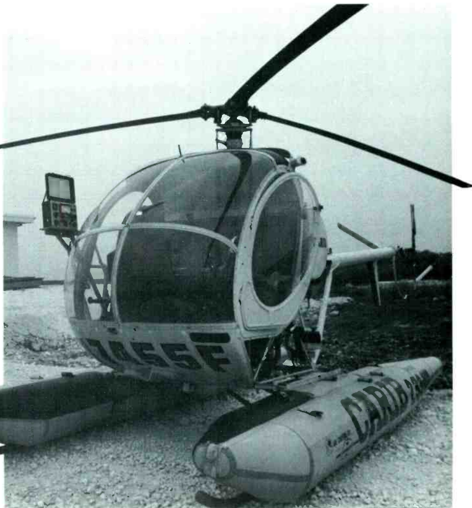
Special test equipment bracket and field intensity meter are shown attached to the helicopter.
