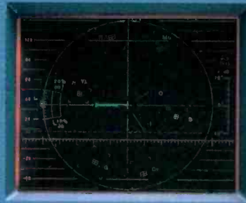
Correct SCH phase relationship is clearly displayed on the 1750 when dot on the calibration circle is aligned with the vector on the -x axis.
