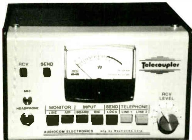
The Telecoupler is designed to interface the telephone to an audio console during two-way conversation such as telephone interviews, telephone talk shows or "on-the-spot" news coverage.
