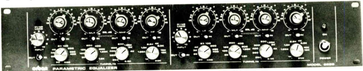
A two channel parametric equalizer for use where continuous, non-interacting control over center frequency, bandwidth, and amount of peak boost or cut is desired. Four peaking bands per channel with "constant-Q" curves
