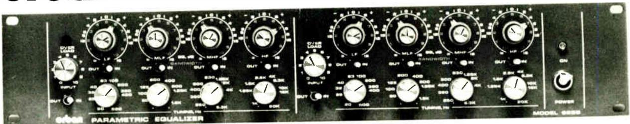
A two channel parametric equalizer for use where continuous, non-interacting control over center frequency, bandwidth, and amount of peak boost or cut is desired. Four peaking bands per channel with "constant-Q" curves
