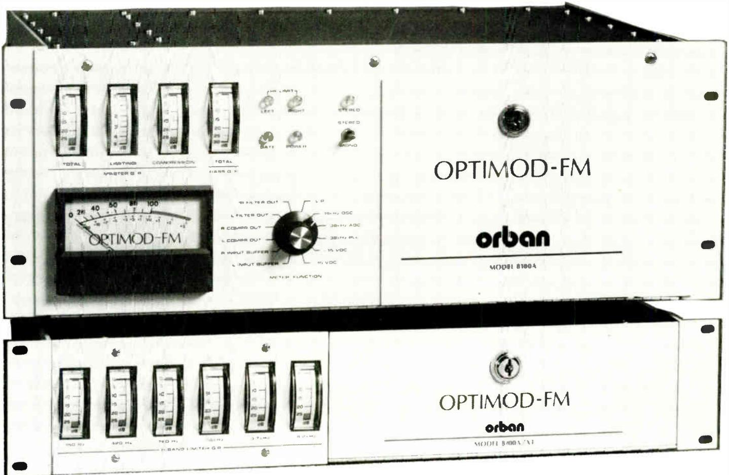
The new Orban 8100A/XT Six-Band Limiter Accessory Chassis for OPTIMOD-FM (Model 8100A) has been created to provide aggressive multiband processing for stations that desire bright, loud, "highly-processed" audio. Derived from the OPTIMOD-AM Model 9100A, the "XT" consists of a six-band limiter cascaded with the exclusive Orban distortion-cancelled multiband clipping system.
