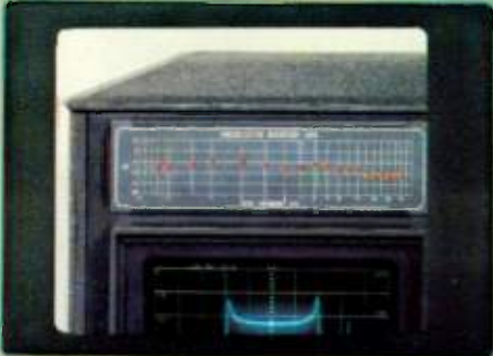
Preselectors in 640A-1 are individually calibrated
