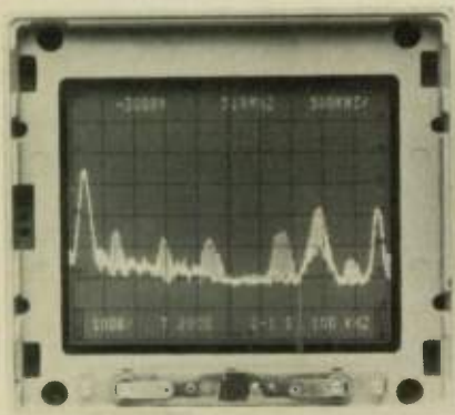
Fig. 1 UHF television signal spectrum displayed by Tektronix 492P Spectrum Analyzer.
