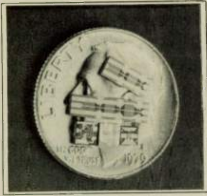
Fig. 4 Photograph of MMIC broadband amplifiers and receiver front end component chips.
