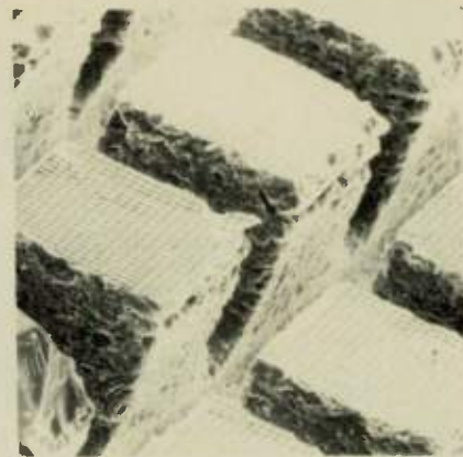
Fig. 2b Electron photomicrograph of notch front diodes.
