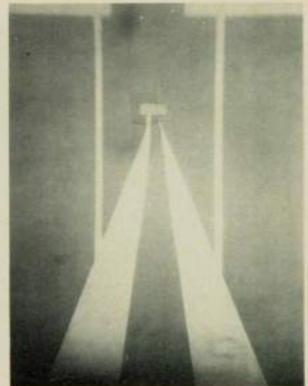
Fig. 7 Integrated Schottky diode/antenna structure for \lambda = 1 mm. Photo courtesy of G.-G. Iau.
