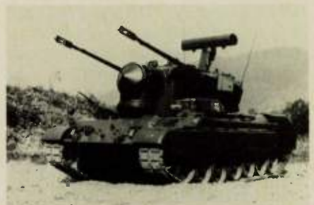
Fig. 18 Flakpanzer AA tank for the Dutch Army, showing X-K a -band tracker in front (photo courtesy Hollandse Signaalapparaten).
