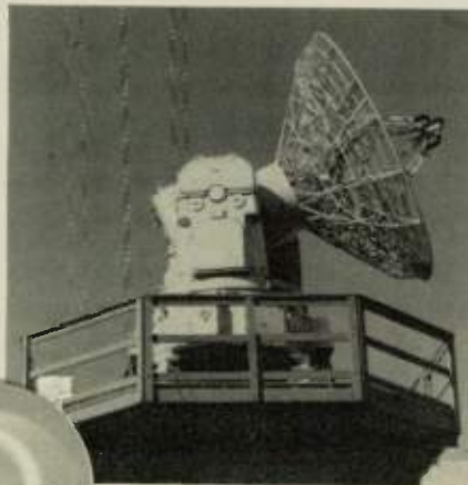
Fig. 9 Monopulse radar for guided missile range instrumentation, the AN/FPS-16 (photo courtesy RCA).
