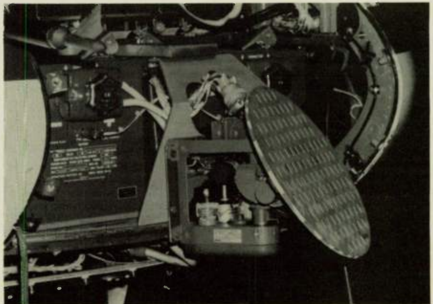
Primus-400 12" antenna installed under radome of Bell 121.
