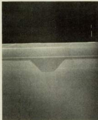
Fig. 4 SEM photograph of DCC laser structure (5000X).
