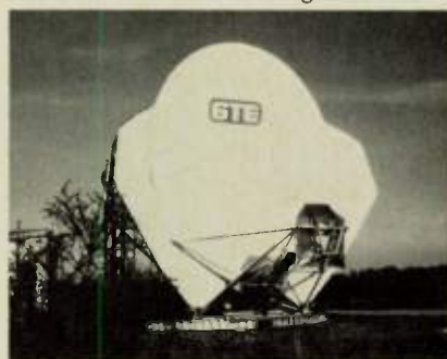
Fig. 10 Low sidelobe antenna - final configuration.
