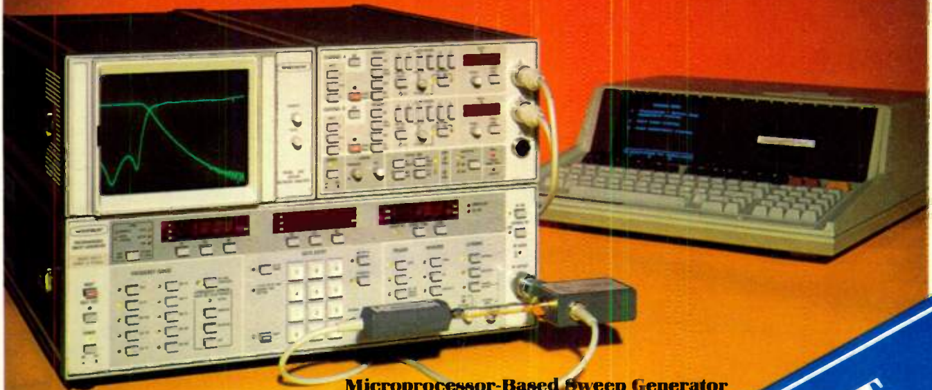
Microprocessor-Based Sweep Generator for Scalar Network Analyzer System
