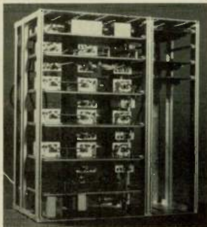
Fig. 8 Receiver unit of the tracking receiver (Electrical model).
