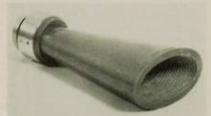
Fig. 5 Elliptical corrugated feedhorn (Electrical model)
