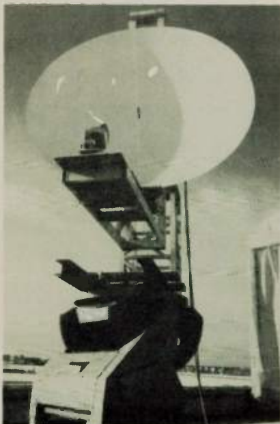
Fig. 4 Reflector with feedhorn (test set-up).
