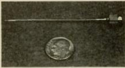
Fig. 1 Microwave syringe (needle antenna) constructed in semi-rigid coaxial waveguide.
