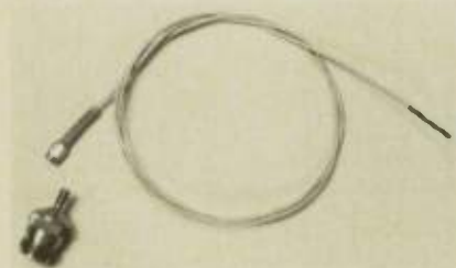
Fig. 2 Microwave needle antenna (coaxial cable form) used in brain cancer therapy.
