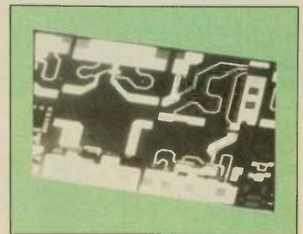
Fig. 9 Scanning electron micrograph of 8 GHz MMIC receiver front end chip.
