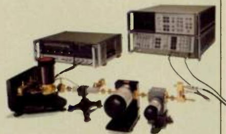
Combination of Hughes (Model 4743xH Series) External Mixer and Hewlett-Packard 8566A Spectrum Analyzer.
