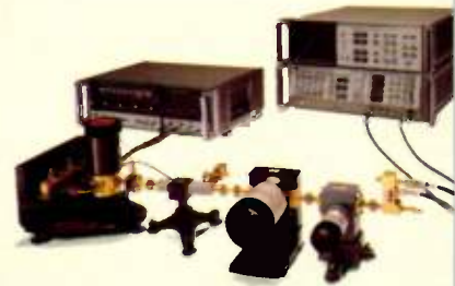
Combination of Hughes (Model 4743 xH Series) External Mixer and Hewlett-Packard 8566A Spectrum Analyzer.
