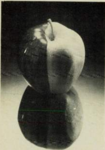
Fig. 3 Zinc with 770°F melting point can be sprayed on any substrate without overheating.
