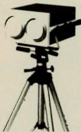
Fig. 9 94 GHz FSK radar mounted on tripod for field test.
