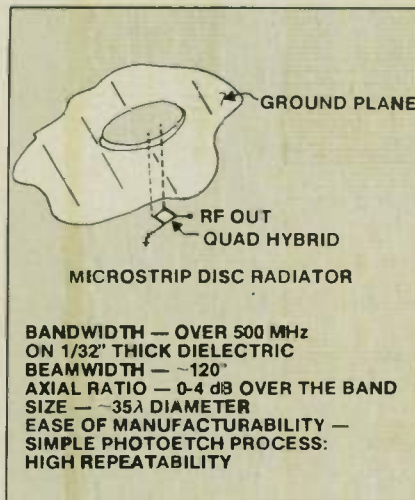
Fig. 1 Microstrip disk radiator.
