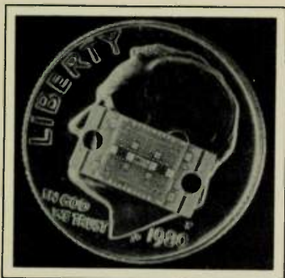
Fig. 2 A 4-12 GHz dual FET amplifier with complete bias and matching circuit.
