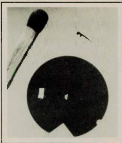
Fig. 3 Disc of the slow wave structure with graphite damping wedge.
