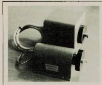
Fig. 7 Backward wave oscillator RWO 170 compared with previous focusing design BWO.
