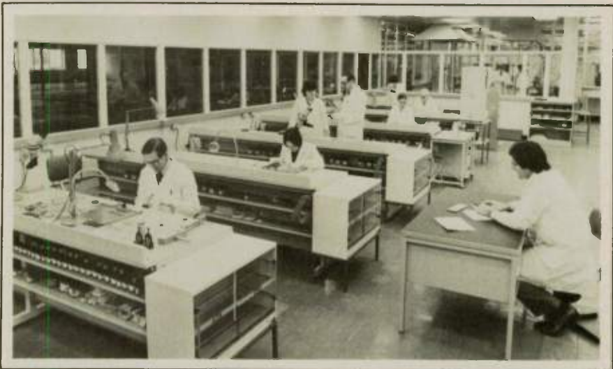
The helix TWT assembly area of EEV's tube facility at Witham.
