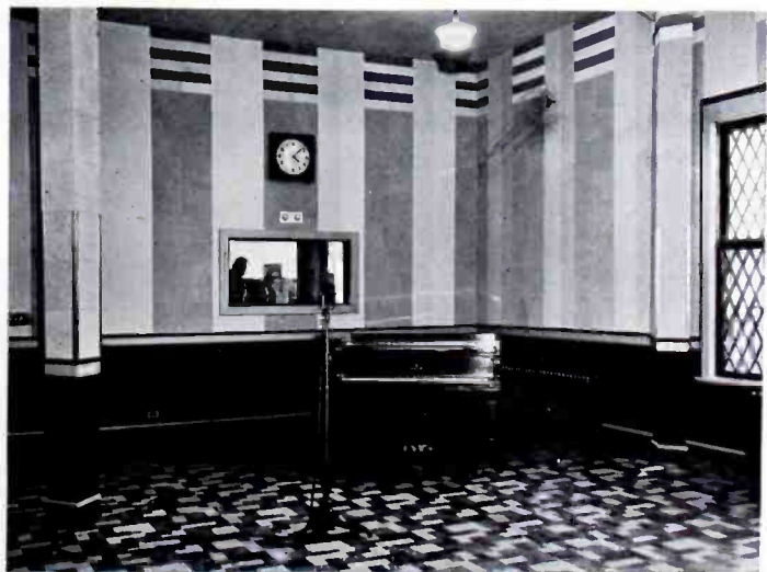
THROUGH THE TRIPLE-PLATE GLASS SOUND-PROOF WINDOW IS THE ORGANIST'S ROOM, WHERE THE PROGRAM MAY BE HEARD ONLY THROUGH A MONITOR LOUDSPEAKER. THERE THE MONITOR OPERATOR (WITH HIS CONTROL EQUIPMENT) IS ALSO LOCATED, CLOSE TO THE ORGAN CONSOLE
