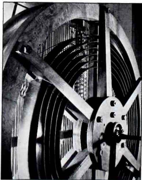
INTIMATE VIEW OF TRANSMITTER INDUCTANCE —TOO INTIMATE WHEN THE POWER IS ON!
