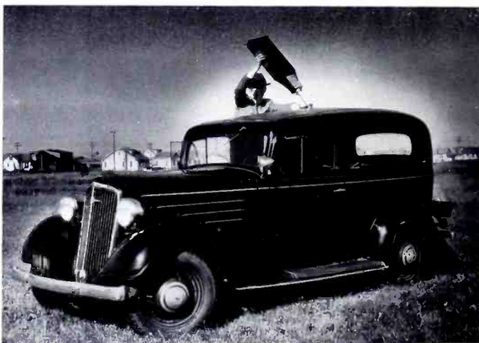
ONE OF THE NBC RADIO ENGINEERING CARS IN WHICH THE RCA TYPE 75-B MEASURING SET, RECORDERS, ETC., HAVE BEEN INSTALLED. NBC USES FIVE OF THESE CARS, SIMILARLY EQUIPPED
