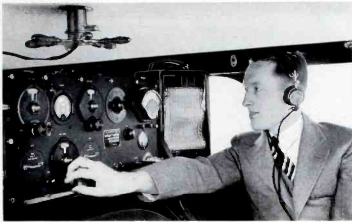
VIEW INSIDE ONE OF THE NBC RADIO ENGINEERING CARS, SHOWING ONE OF THE FIELD SURVEY MEN OPERATING THE RCA TYPE 75-B MEASURING SET. THE GRAPHIC RECORDER MAY BE SEEN AT THE CENTER OF THE PICTURE, AND OVERHEAD IS THE WHEEL CONTROLLING THE LOOP ANTENNA
