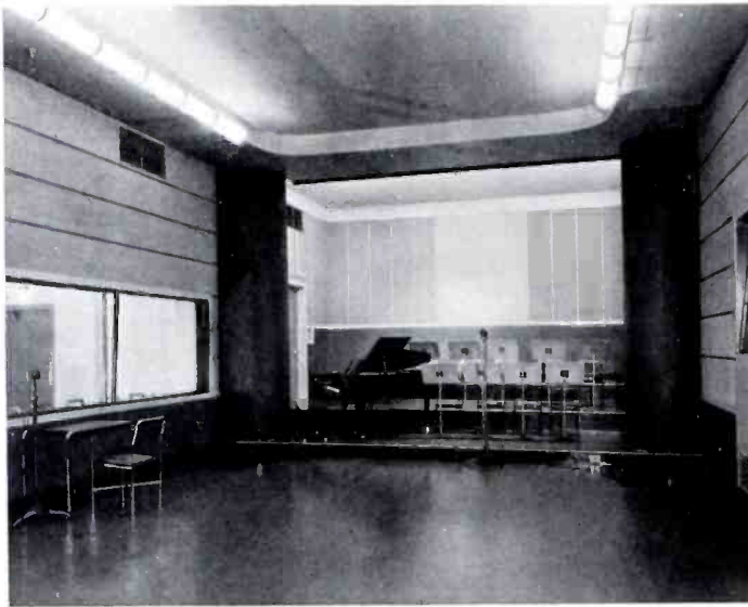
THE CASCADE PLATFORM IN STUDIO NUMBER 3 IS DESIGNED FOR ORCHESTRAL SET-UPS AT STATION WIP. RCA INDUCTOR MICROPHONES ARE EMPLOYED IN THIS STUDIO
