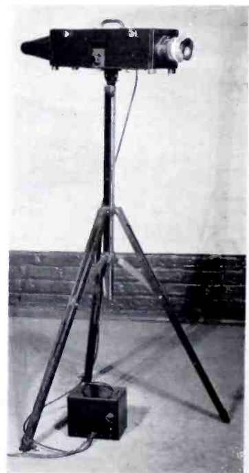
Figure 5. The tube mounted for use as a terrestrial Telescope.
