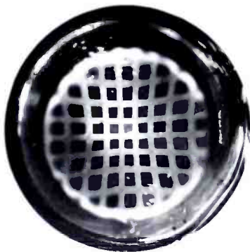
Figure 2. Illustrating the curvature of the image field.
