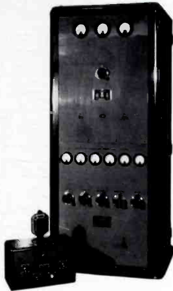
A 100-watt RCA police transmitter which gives excellent coverage.
