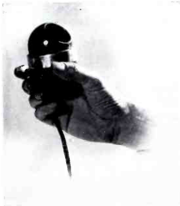
Magnetic microphone for use in the RCA mobile police transmitter ET-5022.
