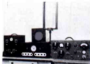
FIG. 14. A setup for making logarithmic recordings. The special linear-logarithmic amplifier shown at the left may be operated either from the receiver or from the recorder direct. It is arranged for either battery or a.c. supply.
