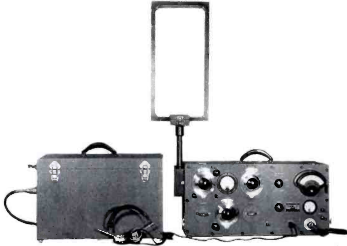
FIG. 1. The new model of the TMV-75-B Field Intensity Meter. Improvements include provision for operating a 5 mil recorder direct.
