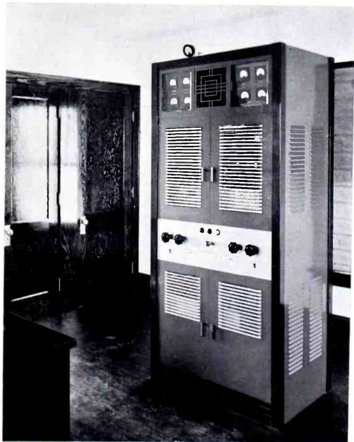
The new RCA ET-4250 Transmitter which steps up power for WRAK.
