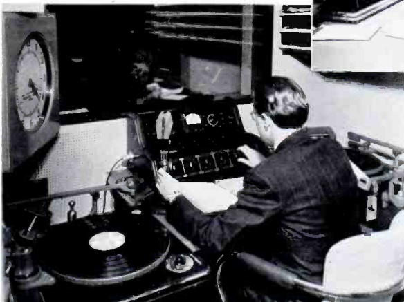
ABOVE: Transcription and Announcement Studio No. 6, showing 70-A turntable, 71-A vertical pickup, and 72-B recording attachment.
