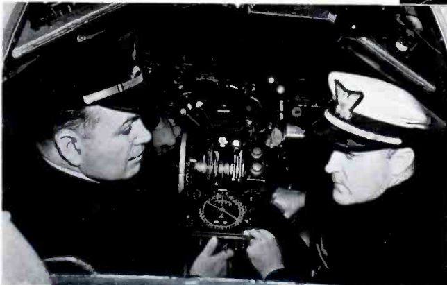
Above: Sperry-RCA automatic direction finder installed in an American Airlines plane.
