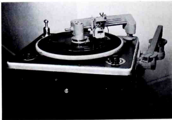
Below: The RCA 70-B with pick-up on the side and the 72 B recording mechanism in position.
