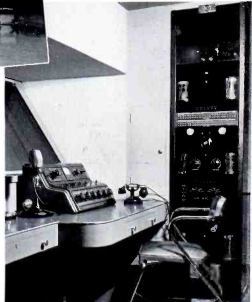
LEFT: In addition to the CBS network control facilities, WCCO Master Control also contains two complete RCA 78-C studio equipments.
